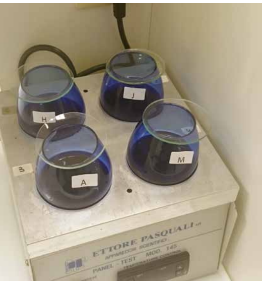
Figure 2. The Tasting Panel. Tasting glass heater. Photo: F. Xavier Vicens Burgués.
